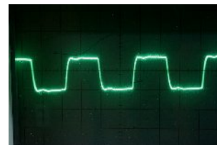
Fig.3 Square Wave 20KHz
